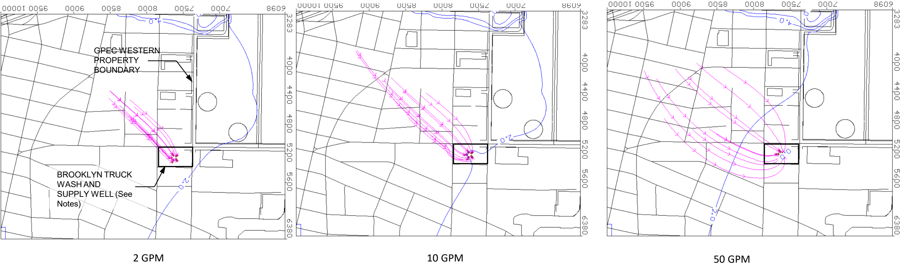
CAPTURE ZONE AS FUNCTION OF PUMPING RATE SUPPLY WELL AT BROOKLYN TRUCK WASH
